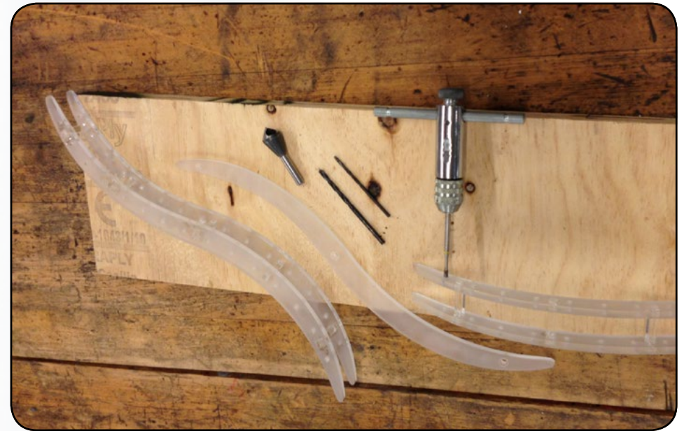
Img 22.2 Threading of the holes to allow assembly with bolts.
