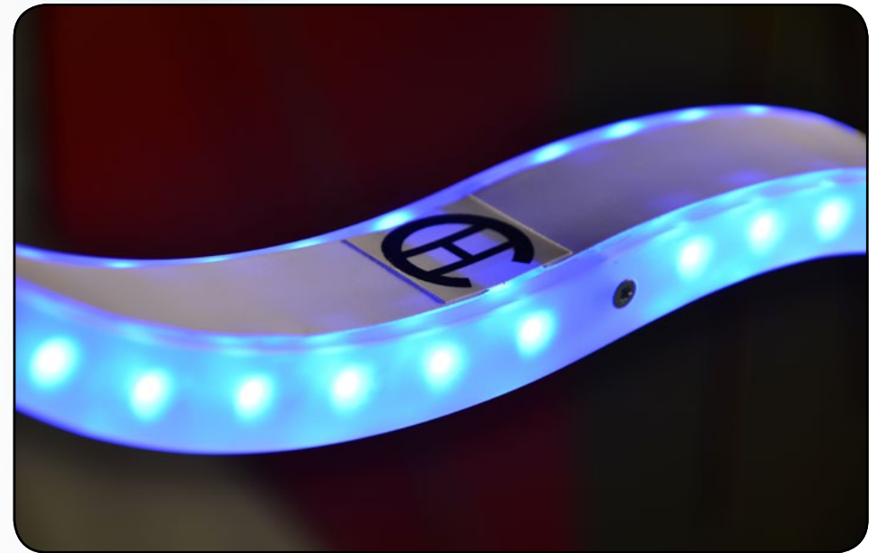
Img 22.3 Final assembly of the parts, with the HC logo to cover the gap.
